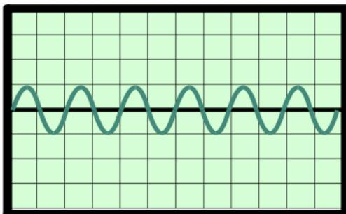
A **quiet** sound on an oscilloscope
